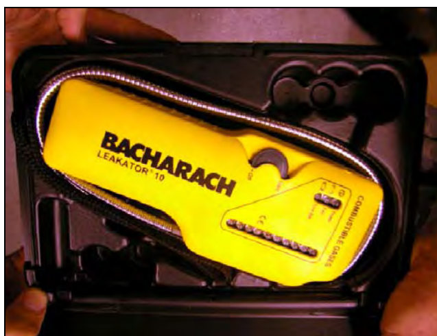
Figure 29. Hydrogen Leak Detector
